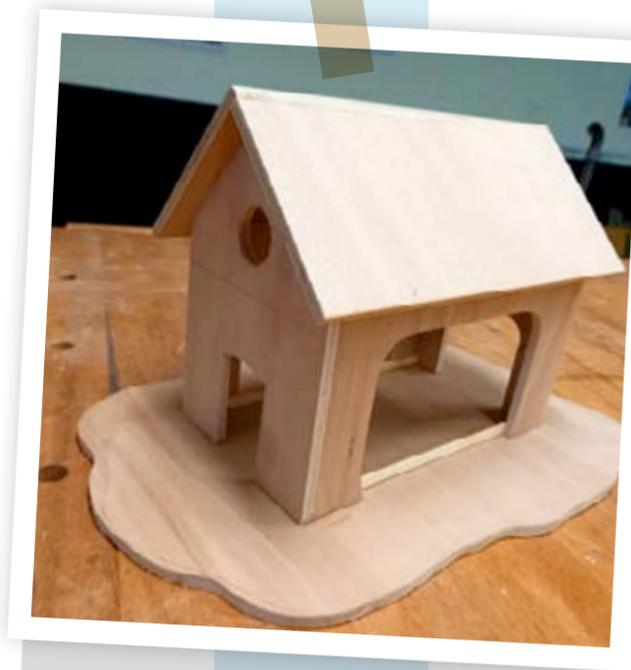
**5** Glue the roof parts together then nail them together. Adding some small strips along the base prevents bird feed from spilling off down onto the ground.
